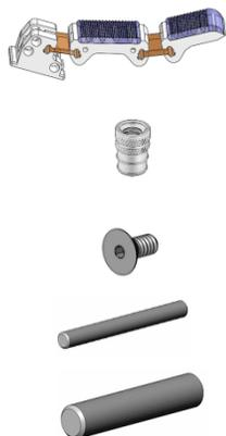
Press fit the 1/8" dowel pins for tendon-rerouting into the proximal link. Press fit the 1/4" dowel pins in the base of the fingers. If the pins do not press-fit easily, use a larger reamer to clean out the pin clearances or a vice. Use a soldering iron to install the heat-set insert into the distal link. The heat-set insert can be skipped in favor of using a nut for tendon termination.
