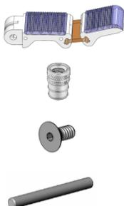
Press fit the 1/8" dowel pins for tendon-rerouting into the proximal link. Use a soldering iron to install the heat-set insert into the distal link. The heat-set insert can be skipped in favor of using a nut for tendon termination.
